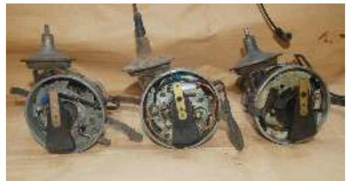
The insides of three different distributors. On the left a single point distributor, in the middle a twin point version and on the right a distributor fitted with Piranha optical (electronic) ignition.
