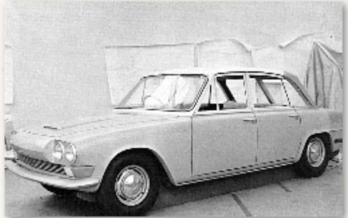
An early wooden model of the new Barb idea. Interestingly, the twin lights within a frontal scoop idea was recycled by Michelotti and the photo shows some claywork on the rear C-post where Triumph styling staff have made some small alteration to the body lines.
