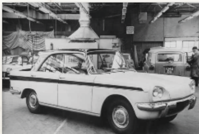
The Zebu idea reworked with a conventional rear window (X743) but still with a pillarless body and with twin headlights, again seen in the Engineering Department workshops.
