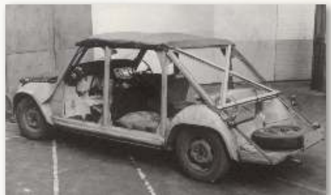
The 'Birdcage', as it was known, with which the Engineering Department carried out the initial endurance testing for the new large saloon. Believe it or not, this was a road test vehicle and spent not a few hours being driven over the company's normal test routes
