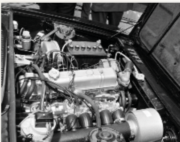
Taken at the Motor Show, this picture shows the straight six PI engine in-situ. The injectors feed into the inlet manifold just before the inlet ports, the fuel lines disappearing down the far side of the cylinder head to a high pressure pump located on the side of the crankcase.
