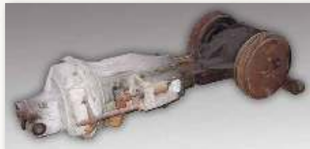
The Transaxle idea which combines the gearbox and differential at the back. Are those inboard brakes on the sides of the diff, or am I imagining things? (Photos courtesy ArchivioStoricoMichelotti, Martin Cox, Canley Classics)
