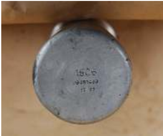
The base of the above coil showing the stamped model and part numbers (15C6 and 45243B).
