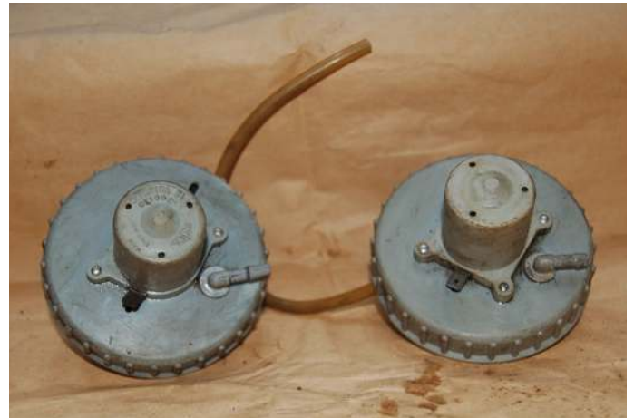
The late cap and pump on the left (two rivets) and the early cap on the right (four rivets). The connection terminals are located at the base of the pump for both pumps.
