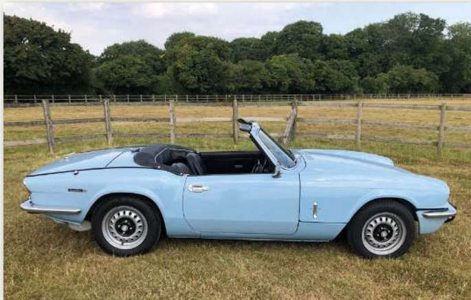
Probably the classic view of a Spitfire. This is a mk4 with standard steel wheels and the new inset door handles.
