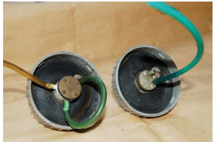
The underside of the two different washer caps, the earlier type on the left and later on the right. The pumps are similar but have input and output nozzles in a different plane - the earlier out of the side and later out of the bottom.
