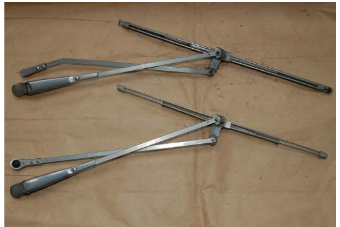
The two pantograph arrangements for the driver's side wipers – one straight and one cranked. The cranked one here is incomplete as it should have a pivot knuckle at the base of the pantograph and it is missing because I broke it off when removing it for the photo.
