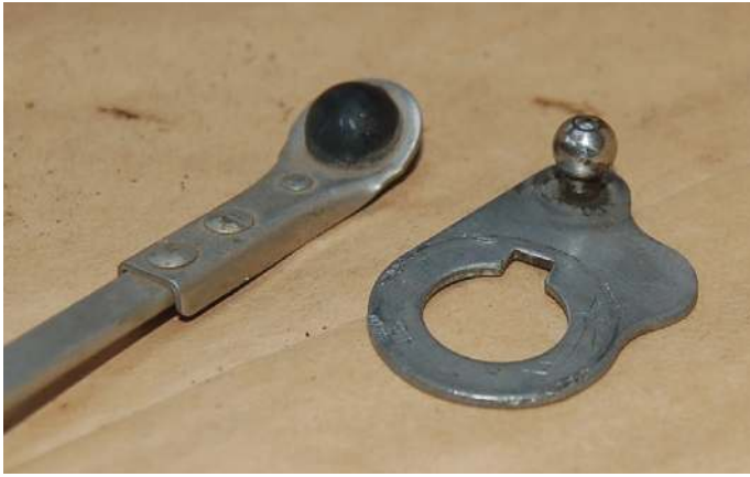
The end of an early (straight) pantograph arm and the stainless ball plate for the pantograph bush to locate on. There is apparently no part number for this plate as the parts catalogue is 'confused' on the subject.
