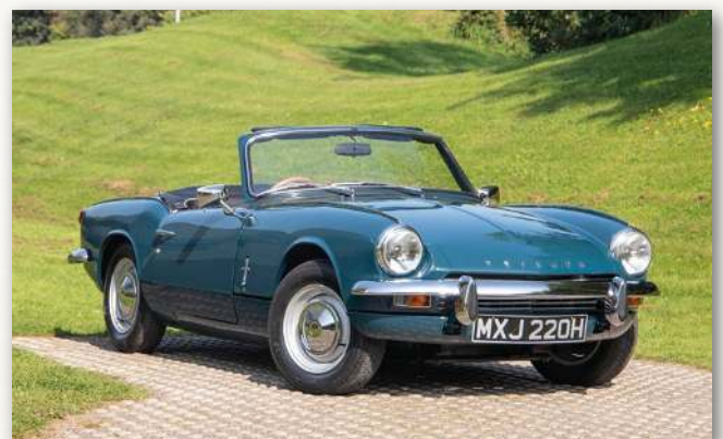
For 1967, the front bumper was raised to give a lower look to the front end, which was revised with a full width grille and under-bumper indicators/side lights. A larger version of the SC engine was also introduced.
