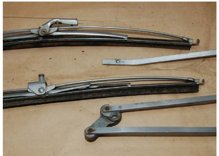
The 'normal' passenger side wiper blade holder and blade (top) and the 'special' driver's side wiper blade holder and blade (bottom). Other blade holders do not have the special fitting for the pantograph type arm as they have the 'normal' fitting on the driver's side as well.
