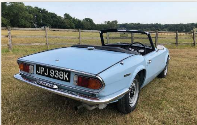
And from the back the Mk4 had the new 'Triumph look' with a cut-off tail and block lights.
